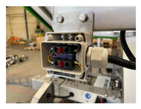
6) In the right side of the robot, cut the zip ties and pull about 15 cm of the cable running to the HMI, fix the extended wire with two zip ties
