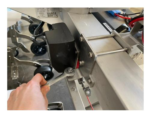
15) Secure the left-side bracket of the power bank to the frame, using 5 screws. Make sure to tighten the nuts.
