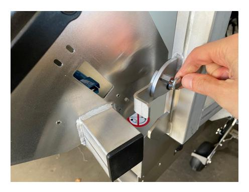
21) Then tighten the bolts on the other side. These bolts should be tighten only AFTER closing the power bank case, to make sure all components are aligned.
