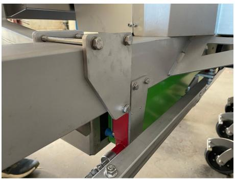
11) Have a person to hold the power bank assembly in place, then tighten the two screws which secure the assembly to the top part of the robot's frame
