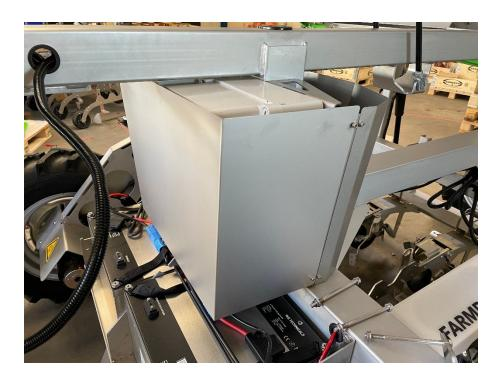
5) Remove the emergency stop by using a screwdriver and a 3mm Allen key
