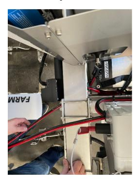
19) Plug in the cable on the available plug, placed in the left side of the battery housing
