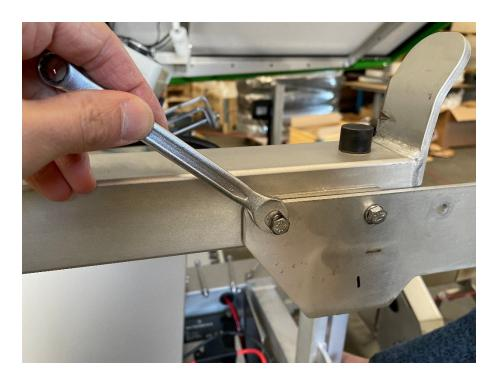
9) Now secure the lower part of the bracket to the robot frame
