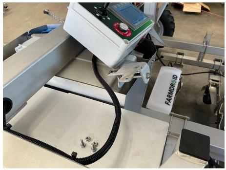
8) Secure the power-bank side support bracket to the upper part of the frame. NOTE: you may need help from another person to hold the bracket in place.
