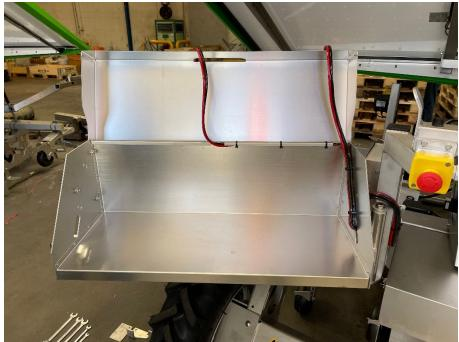
25) Place the batteries in the case and connect them to the robot
