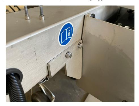
3)Remove the old actuator support, in the left side of the robot
